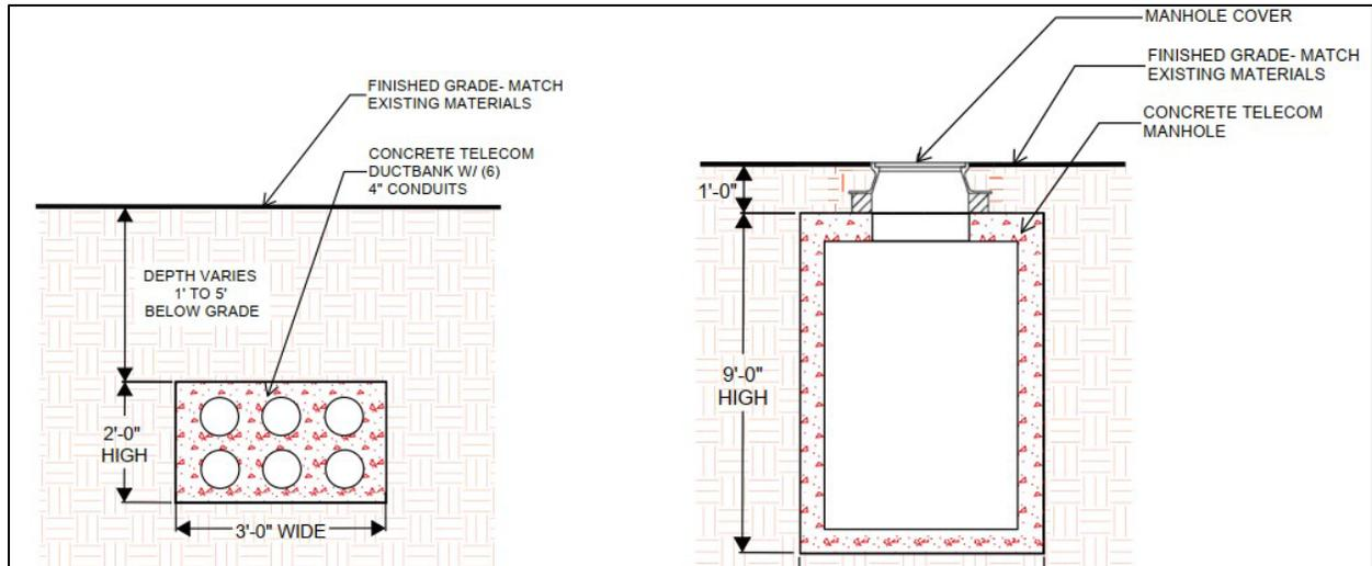
Detail sections of the Telecom Duct Bank and Manhole Access.
