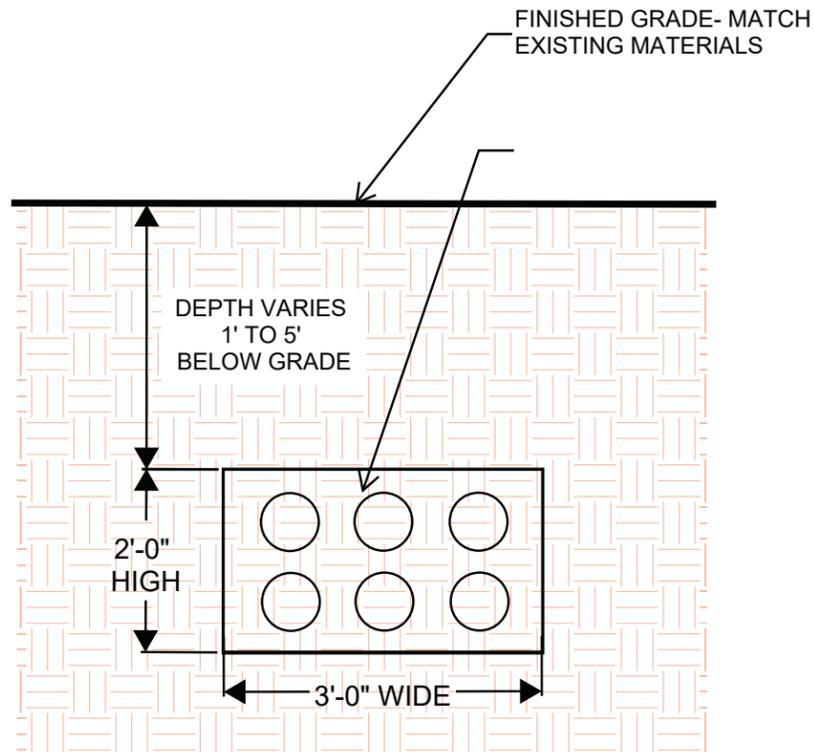
Figure 1.1.3.b - Detail section. Proposed new telecom ductbank.
