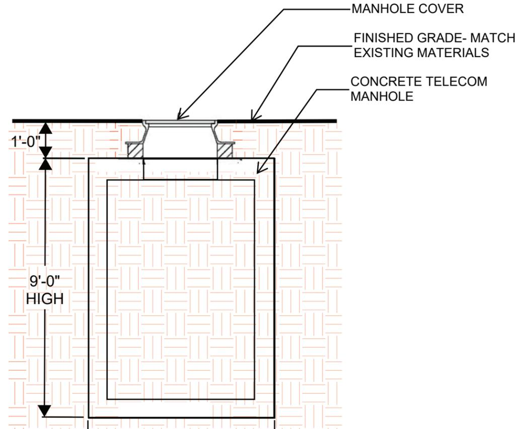
Figure 1.1.3.c - Detail section. Proposed new manhole.
