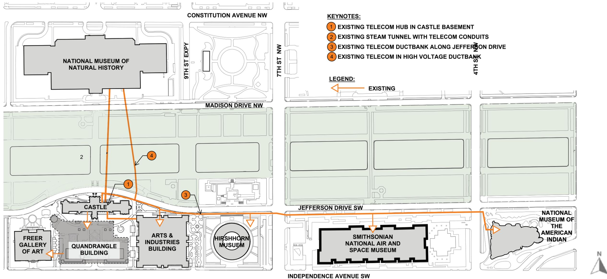
Figure 1.1.1.a - Site plan. Existing conditions diagram.
