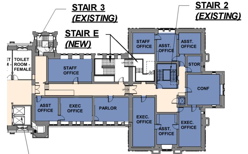
3<sup>rd</sup> Floor, Internal Stair Analysis. Stair E is a new insertion that would impact a historic room on this level and each other level down to the Basement.
