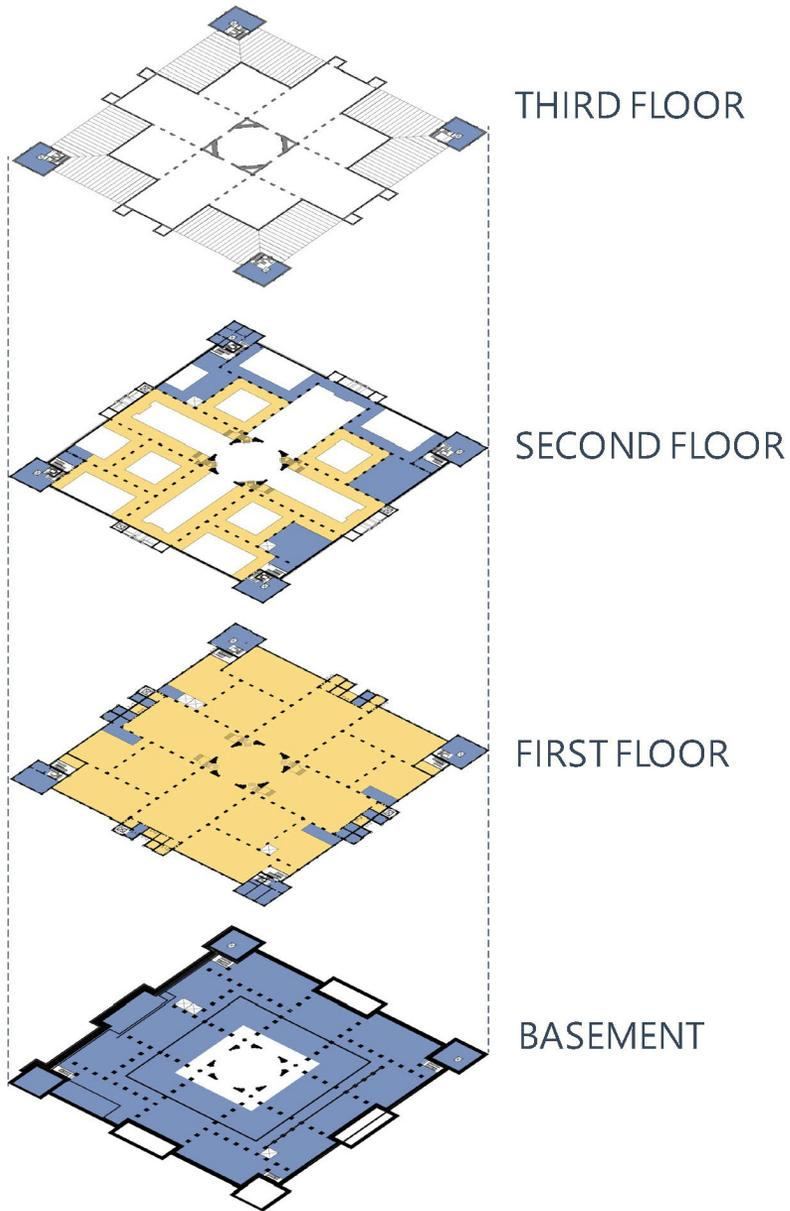
The new basement level will create space for mechanical/electrical equipment and support space for Smithsonian staff. This will allow the historic spaces on the 1st and 2nd floors to be utilized primarily for public functions.
