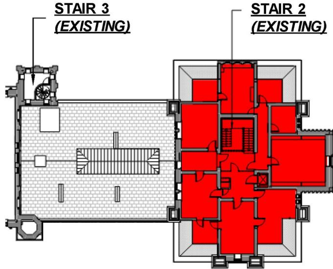
4<sup>th</sup> Floor, Existing Condition Plan. Red indicates the portion of the floor that cannot be occupied by code without an additional means of egress.
