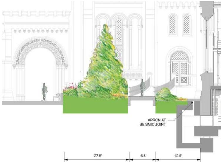
Proposed Seismic Control Joint - North
